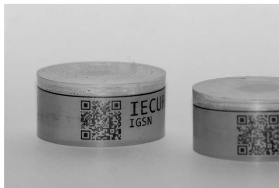
Figure 2: Mineral mounts with embedded QR codes
